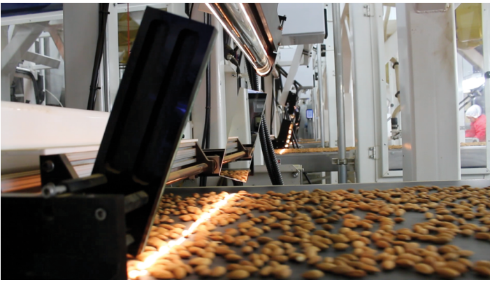
Figure 9. Optimized broadband lighting allows the highest quality hyperspectral imaging data to be captured. Important considerations include uniformity of coverage, wavelength range, and robust construction.
